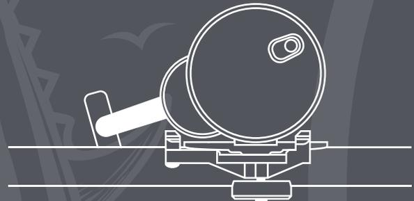
**Step 3:** Slide the adjustable crossbar over the front of the reel seat as close to the reel as possible. Tighten screws "A" evenly. Then align the assembly with the rod guides and tighten screws "B" evenly. Be sure not to over tighten.
