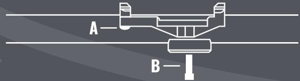
**Step 2:** Set the reel on the rod and position the rear reel seat beneath the fixed crossbar of the clamp.
